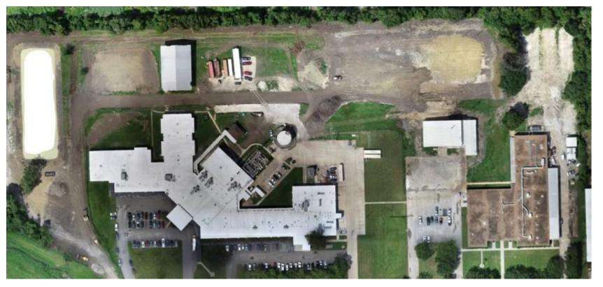
Overall Site - The new roof has been completed on the West Building of the campus, the detention pond has been dug, and the layout of the road around the west side of the West Building and to the north of the building has been cut. Work is continuing at the north parking lot. Openings have been built into the new cafeteria area for windows and glass doors.
