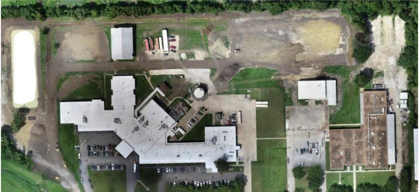
Overall Site - The new roof has been completed on the West Building of the campus, the detention pond has been dug, and the layout of the road around the west side of the West Building and to the north of the building has been cut. Work is continuing at the north parking lot. Openings have been built into the new cafeteria area for windows and glass doors.
